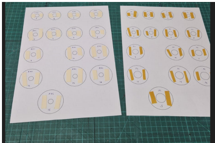
(a) PTFE rings (in figure placed on a sheet of paper) before being located in the prepreg, one per each interface
