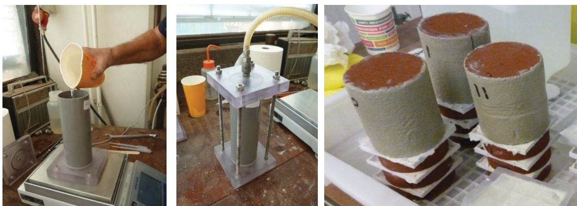
Figure 7. Pouring of the product in the PVC tube (left), application of the pressure (middle), testing of actual effectiveness of the product on a layered structure of brick and clay
