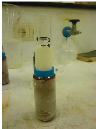
Figure 3 left. Impregnation of brick cores by hydrostatic pressure (left) Figure 3 right. Sketch showing the slicing of brick core and the direction of the water absorption measurements on the three brick parts
