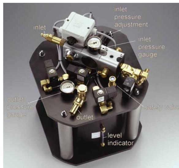
Figure 4.9: The PivPart45 particle generator used to inject the seeding particles, taken from the PivPart45 manual [99].
