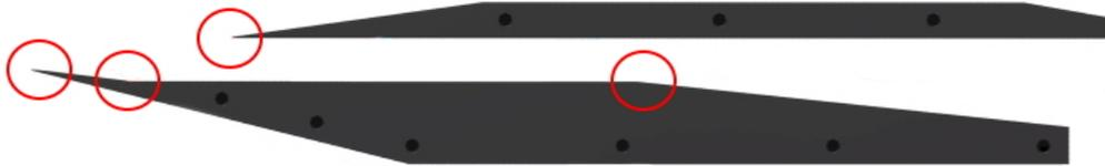
Figure 4.17: Side view of the SSI model featuring the locations with the highest degree of light reflections, indicated with red circles, during the PIV campaign.
