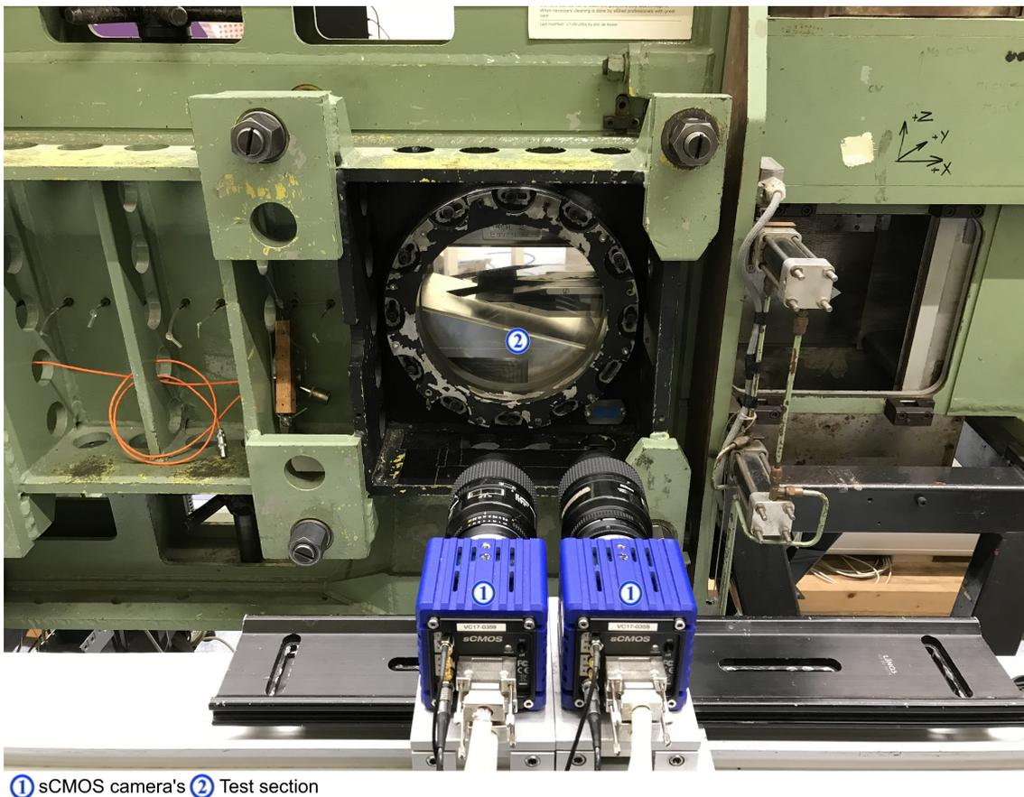
Figure 4.15: Image of the sCMOS camera setup for the PIV campaign.
