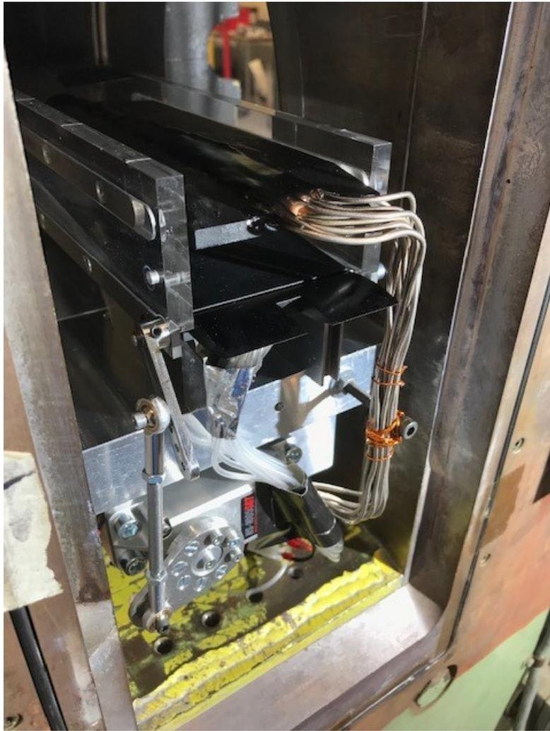
Figure 3.21: Image of the complete actuation system mounted in the wind tunnel, taken from an isometric view.
