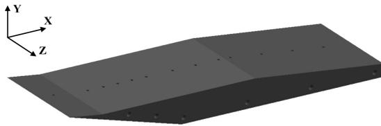
Figure 3.10: Isometric view of the double-shock compression plate.
