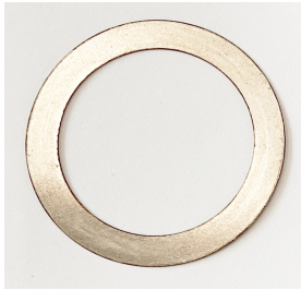
Fig. 7: Laser cut spring steel.
