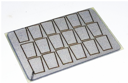
Fig. 8: Laser cut PZT plate.
