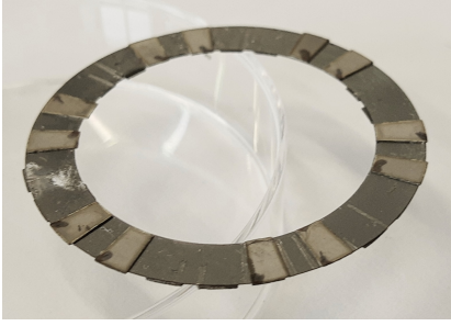
Fig. 11: Prototype ring with PZT elements.
