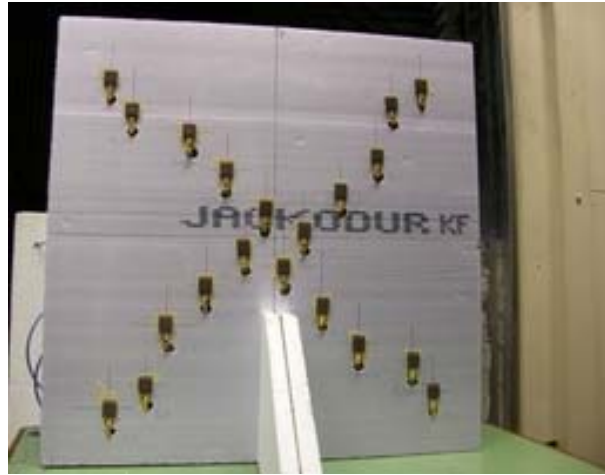
Figure B.1 Example of sparse antenna array for UWB near-field imaging (Courtesy of Yu-Che Yang) [1]
