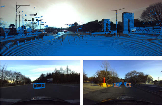
Fig. 5. Visualization of the dataset’s sensor miscalibration (left) and two failure cases of the model. One shows a missing detection of a crossing object (center) and the other shows false negatives for partially occluded objects (right). The ground truth is shown in blue and the model prediction in orange.
