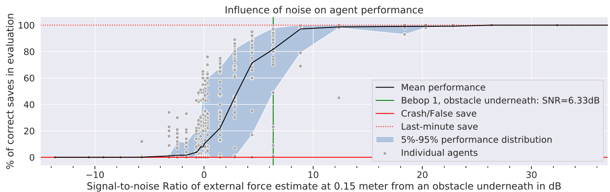
Fig. 13 Influence of noise on agent performance, as measured by the percentage of episodes resulting in a save.
