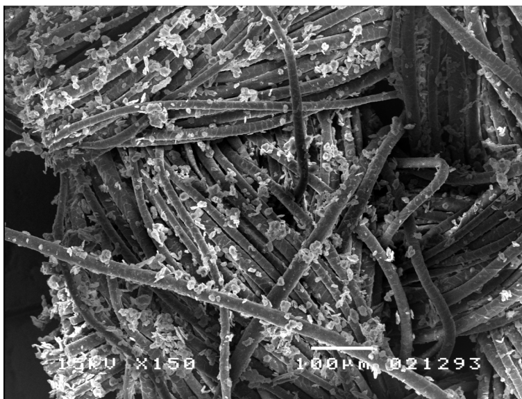
Figure 7: Amihope LL particles deposited at the fibre surface using no mechanical action
