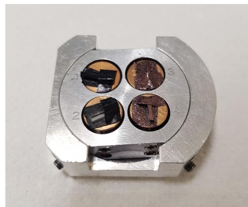
Fig. 9. Prepared samples for SEM.
