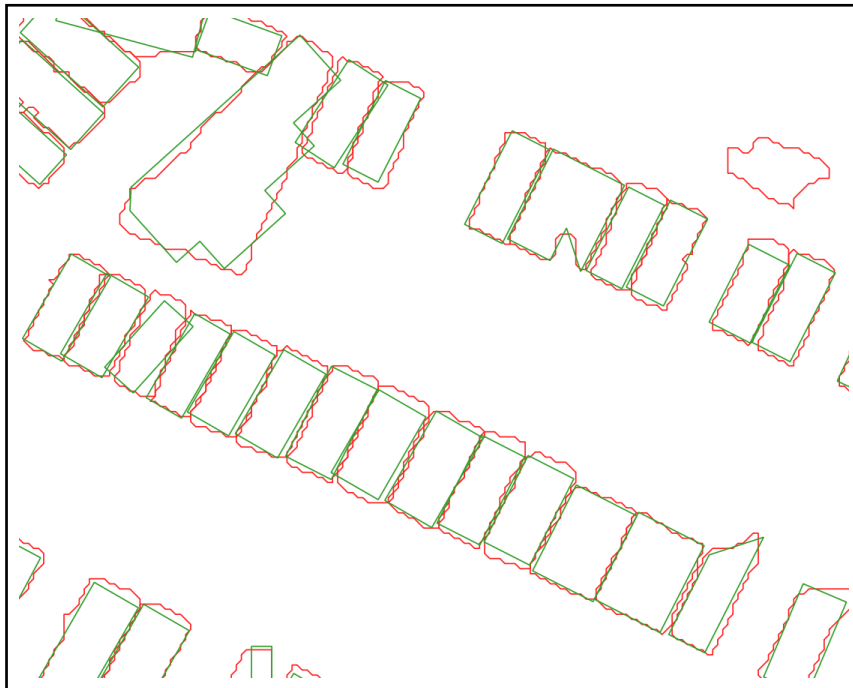
Figure 5.32: Building polygons after post-processing and regularisation, shown in green. Raw Mask R-CNN predictions shown in red for comparison.
