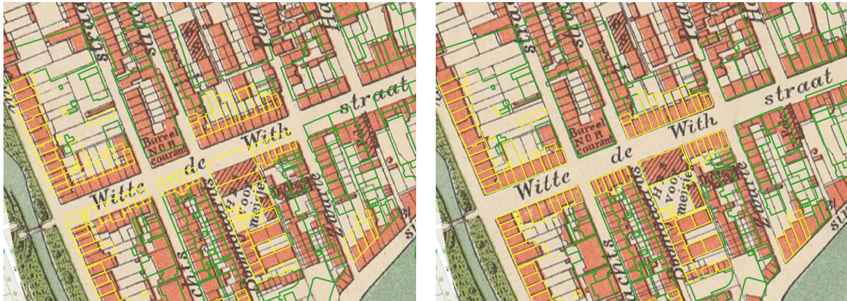
(a) Before: Allmaps annotation. (b) After: Improving the placement of GCPs. Figure 5.15: Overlay of Rotterdam 1897 sheet 3 with BGT Pand layer (buildings with bouwjaar < 1897, shown in yellow outline, buildings with bouwjaar > 1897, shown in green outline) before and after improving placement of GCPs.
