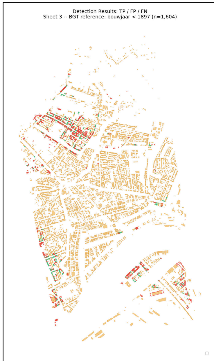
Figure 5.36: Spatial distribution of matching results across Sheet 3. Green: true positive predictions matched to a BGT reference building. Orange: unmatched predictions (FP). Red outline: BGT reference buildings not detected (FN).
