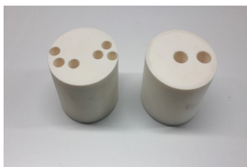
Figure 1: Samples GP.3.4 (right) and GP.4.2 (left) are tested in the impedance tube, using the transfer function method and the standing wave ratio method
