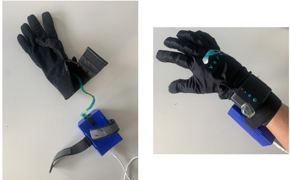
**Figure 2.** Left: Overview of the system (VRFree glove and HD), right: user wearing the system
