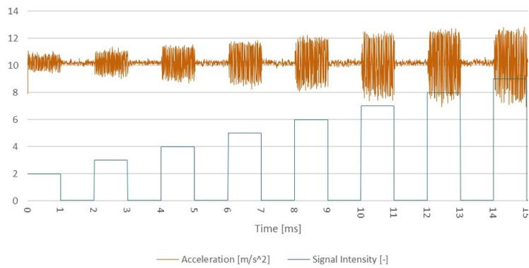
**Figure 7.** Acceleration of LRA during different intensity settings
