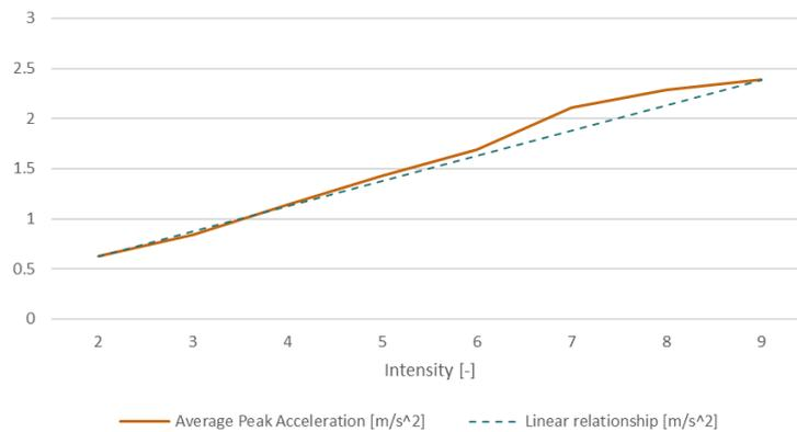
**Figure 8.** Average peak-acceleration of LRA during different intensity settings
