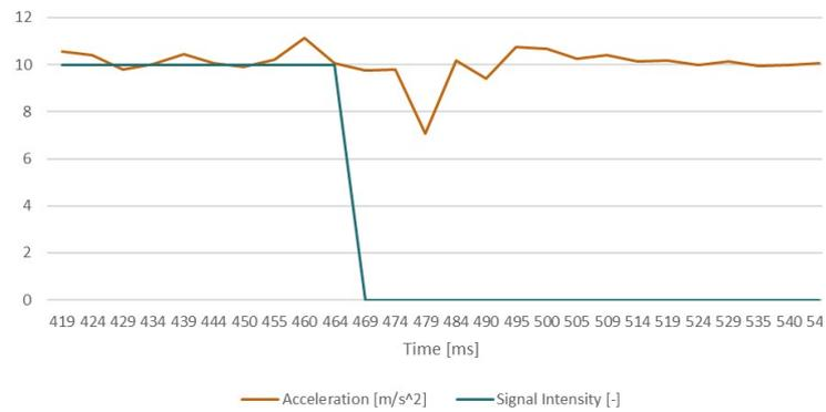
**Figure 6.** Acceleration of LRA on collision stop signal
