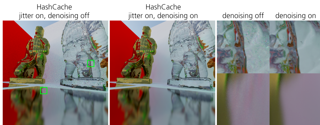
Figure 16. The effect of layered filtering for glossy and specular materials. The cache was filled irregularly over 128 frames at 1 spp for a random fly-through. (Left) Unfiltered image at 128 reconstruction samples per pixel. (Center) Layered filtering at 128 reconstruction samples per pixel. (Right) Magnified insets. It is clearly visible how the noisy illumination from the back wall is reflected in the glossy surface on the ground when layered filtering is deactivated. With layered filtering, the noise can be filtered in a separate layer and then be accounted for in the glossy reflection. For the refractive material on the right, a similar effect is visible: Refracted rays pick up the noisy cache values from the back wall when layered filtering is deactivated. With layered filtering turned on, this noise can be effectively filtered before it is propagated to preceding vertices on the path. This allows for removing the noise locally without loss of details. An example for the individual layers being filtered is shown in Figure 10.
