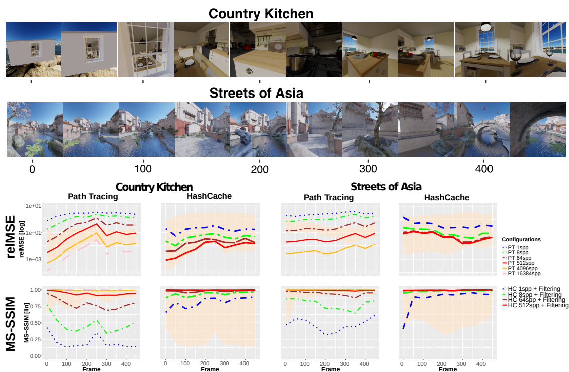
Figure 11. Relative mean square error (relMSE, lower is better) and multi-scale structural similarity (MS-SSIM, higher is better) for the scene Country Kitchen (maximal build resolution 4096^3 ) and Streets of Asia (maximal build resolution 2048^3 ) at various sampling densities using path tracing and the HashCache system. The shaded area in the background outlines the respective relMSE and MS-SSIM ranges for the other rendering method for better comparison.
