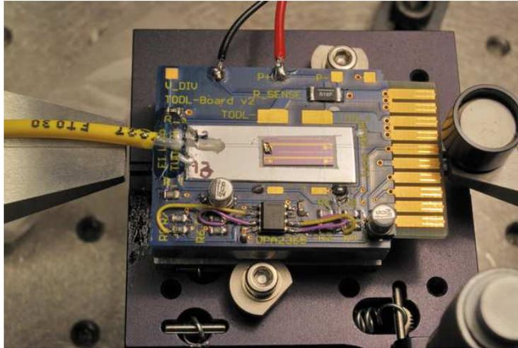
**Figure 4.3.** Aluminium bracket, the TODL-board and a TODL mounted on a rotational alignment stage for fixation of the optical fibre
