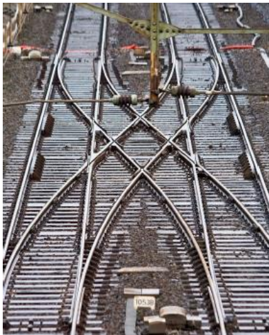
Figure 47: Passing on the switch(es) (Harry Klinkenberg)
