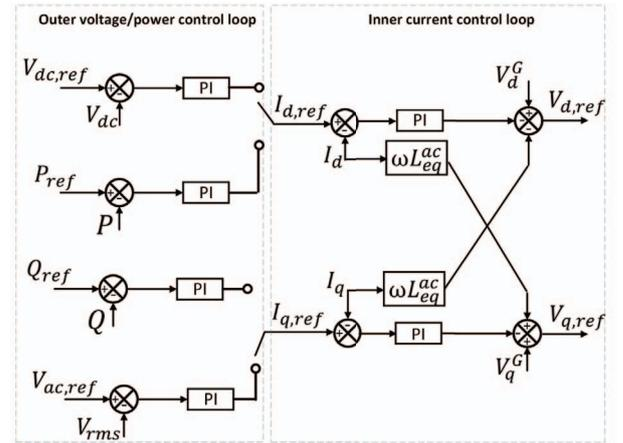
Fig. 2: MMC control for grid-following converters
