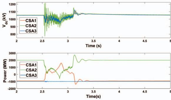
Fig. 10: DC link voltage and active power plots for different MMC's during L-L-G fault using STSMC controller
