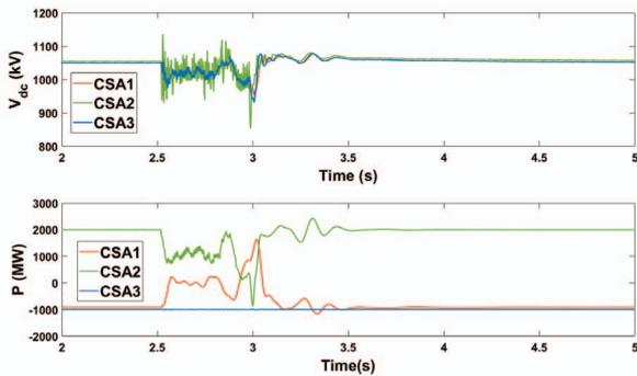
Fig. 11: DC link voltage and active power plots for different MMC's during L-L fault using STSMC controller
