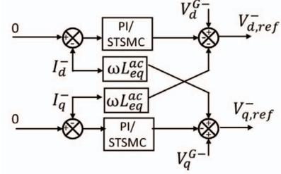
Fig. 5: MMC offshore converter control - Negative sequence
