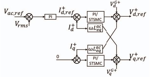
Fig. 4: MMC offshore converter control - Positive sequence
