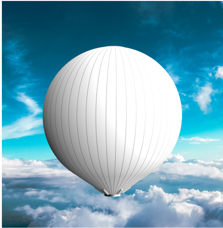
Figure 4.4: A render of the balloon where the vents and load tapes can be seen. Number of load tapes and their spacing does not represent the reality because of hardware limited computing capabilities.
