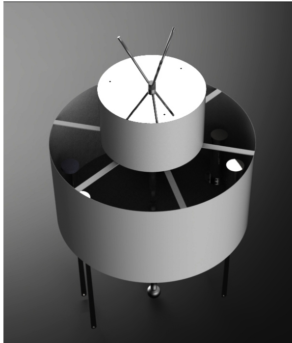
Figure 4.8: A rendering of the preliminary design of the gondola and separation mechanism.
