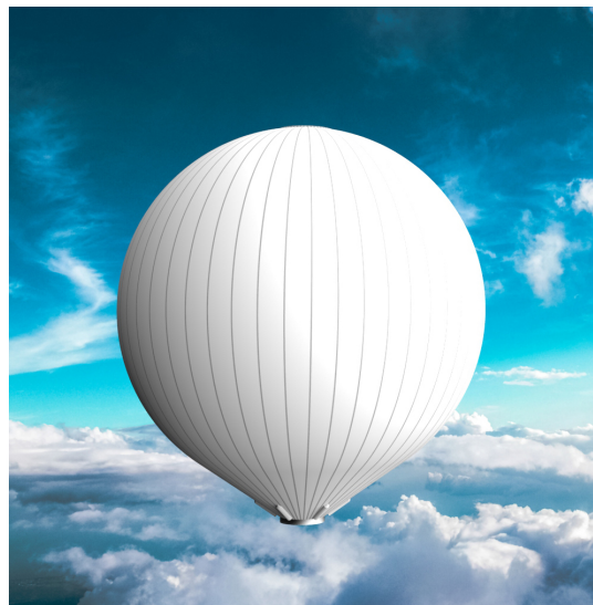
Figure 1: A render of the balloon including the pressure vents, film and load tapes. Fewer load tapes than in reality are shown for clarity.
