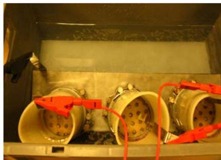
Figure 2: The migration set-up in laboratory
