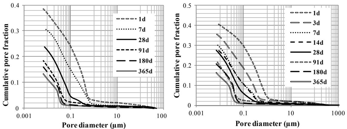
Figure 4: Cumulative pore size of reference sample (left) and the sample blended with 30% FA (right) with a w/b ratio of 0.4 at different curing ages
