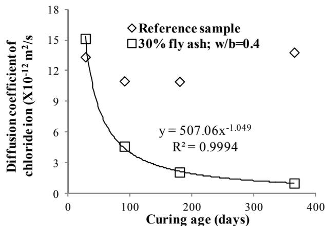
Figure 3: Diffusion coefficient ( $D_{RCM}$ ) of reference concrete and FA concrete
