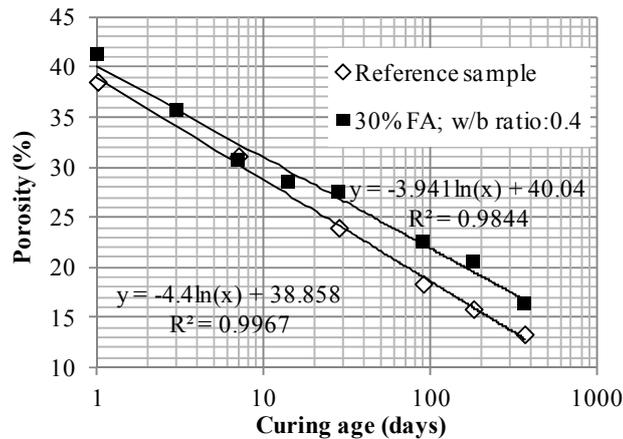
Figure 5: Porosity of reference sample and the sample blended with 30% FA at different curing ages
