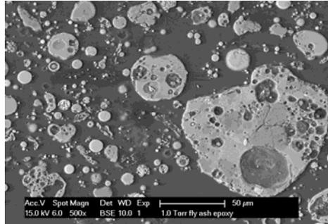
Figure 1: BSE image of FA particles
