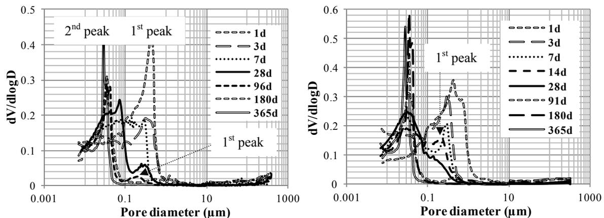
Figure 6: Differential pore size distribution of reference sample (left) and the sample blended with 30% FA (right) with a w/b ratio of 0.4 at different curing ages
