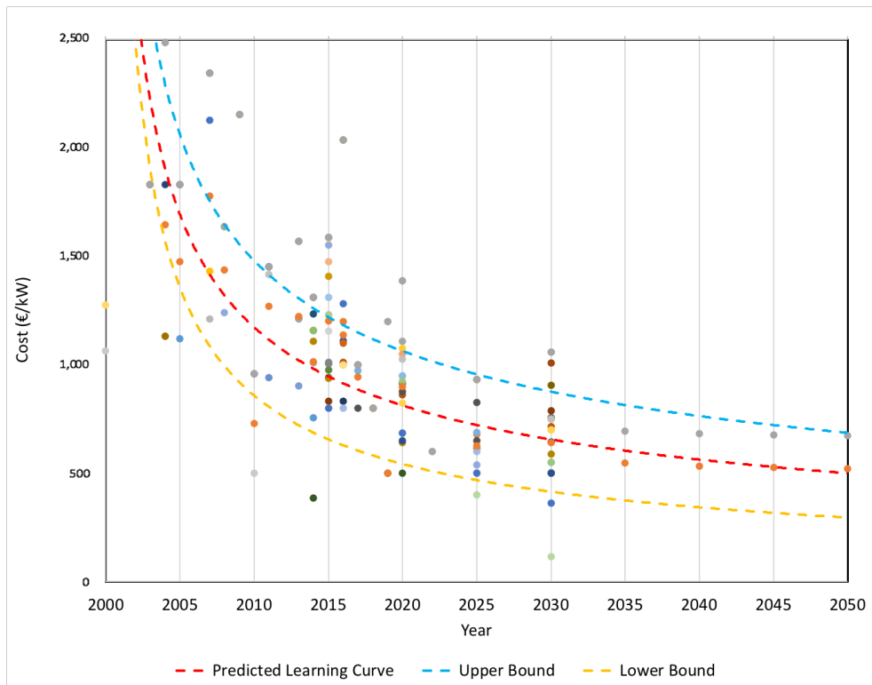
Figure 5.5: The learning curves for alkaline based on future growth prediction. The red is the average predicted learning curve, blue the upper bound and yellow the lower bound.
