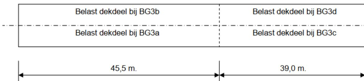
Figure 36. Schematic representation of the temporary load cases
