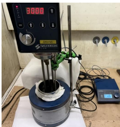
Figure 2-1. shear mixing process with the high shear mixer.
