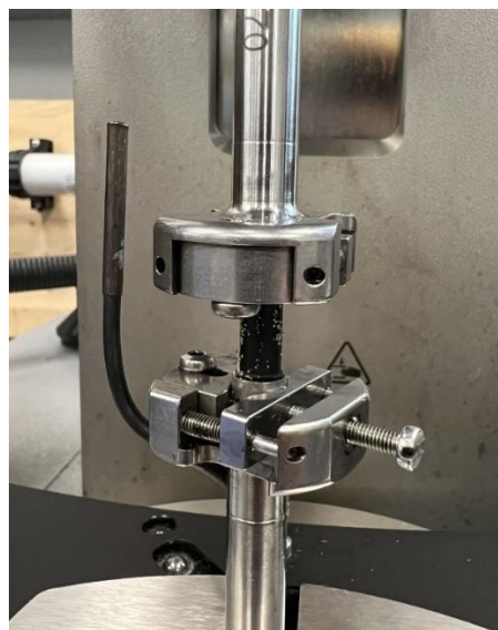
Figure 3-9. Mastic sample in DSR ready for testing.
