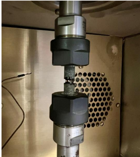
Figure 3-7. Pull-off test with DMA.
