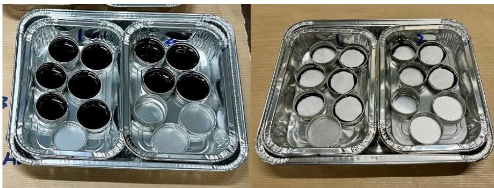
Figure 3-1. Bleeding test samples before (left) and after (right) filter paper was applied.
