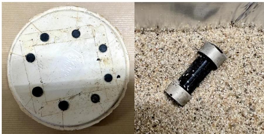
Figure 2-2. (a) Mastic in the silicon mould and (b) de-moulded mastic.
