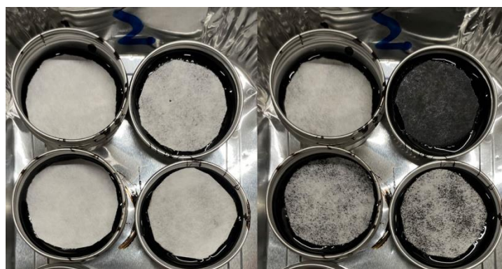
Figure 3-2. Bitumen samples before (left) and after (right) bleeding tests.
