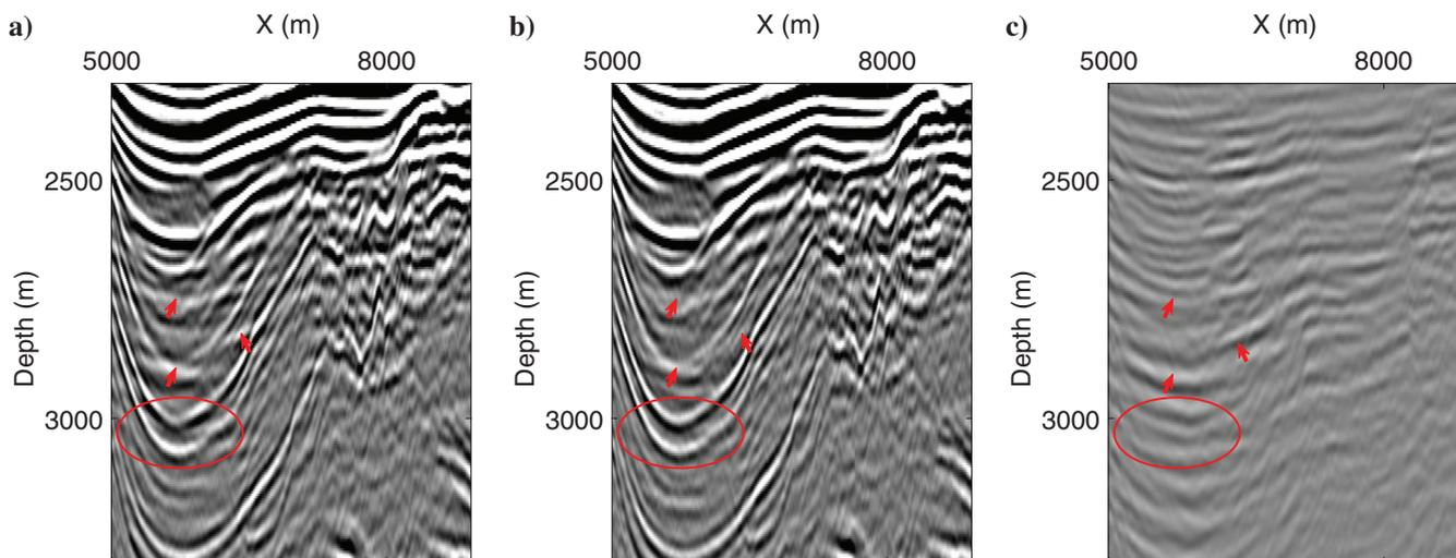
Figure 5. (a) The magnified portion of zone 2 in Figure 3a, (b) the magnified portion of zone 2 in Figure 3b, and (c) the difference between (a and b). The red circle and arrows highlight artifacts due to internal multiple reflections, which are removed after processing by the MME scheme.
