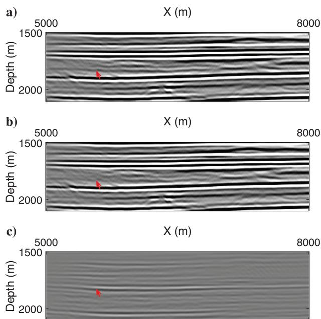
Figure 4. (a) The magnified portion of the zone 1 in Figure 3a, (b) the magnified portion of the zone 1 in Figure 3b, and (c) difference between (a and b). The red arrows indicate the artifact due to internal multiple reflection, which is attenuated after processing by the MME scheme.
