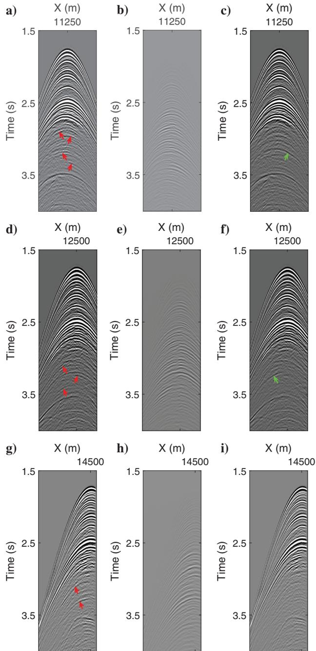
Figure 2. The subparts (a, d, and g) represent the original shot records, (b, e, and h) represent the predicted internal multiple reflections by the MME scheme, and (c, f, and i) represent the corresponding multiple-eliminated shot records. The red arrows indicate internal multiple reflections, and the green arrows indicate primary reflections recovered after the processing.
