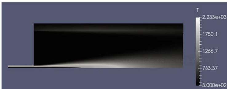
Fig. 2 Contour plot of the temperature (Case 2)
