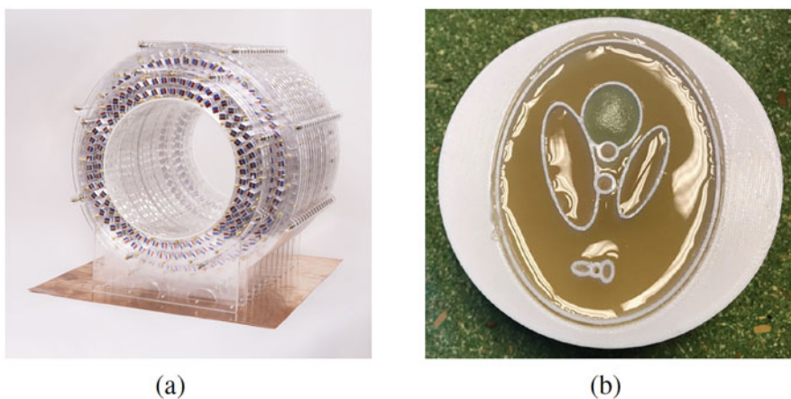
Fig. 2 Experimental setup. (a) Low-field MRI scanner. (b) Object being imaged
