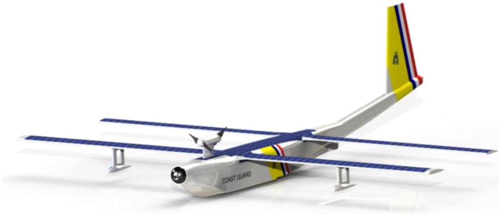
**Figure 1. Illustration of the Dragonfly Unmanned Aerial Vehicle [28]**
