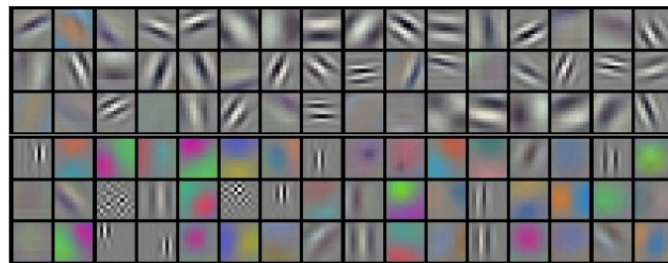
Figure 2-4: The image shows multiple kernels from a filter out of a convolutional layer. This visualization of the kernels gives insight in how a convolutional layer learns to extract features. [3]
