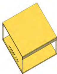
TIMBER HYBRID Utilizing CLT slabs with glulam columns and beams.
