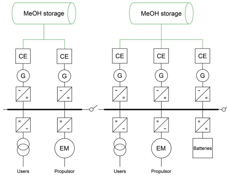
Figure A.4: Potential lay-out of methanol ICE power system
