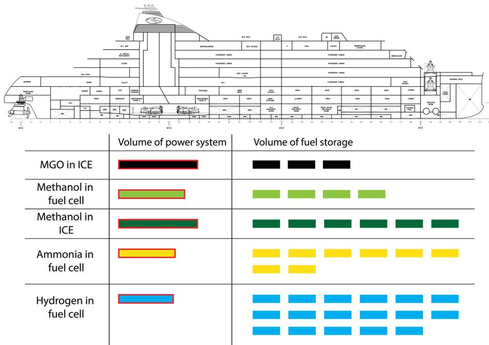
Figure 5.5: Visualization of the volumes of selected fuels and machinery on board of Ship A
