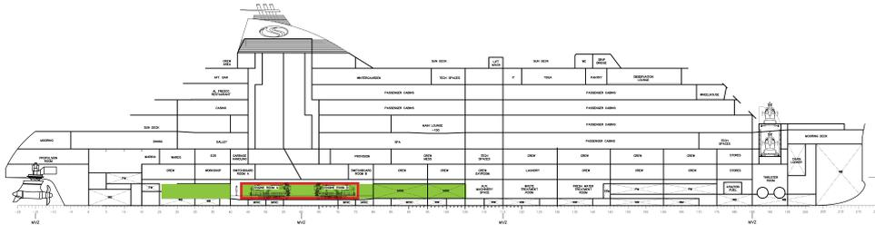
Figure C.4: Schematic GA for Ship A for the methanol FC test case
