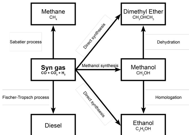
Figure 2.2: Diagram of syngas conversion processes covered in this report, own diagram based on [60]
