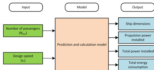
Figure 4.1: Schematic overview of the prediction model
