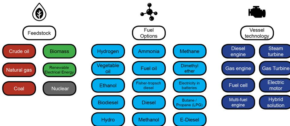
Figure 1.7: Simplified illustration of feedstock (energy source), fuel options (energy carries) and vessel technology (energy conversion) based on DNV [1] and Brynolf [13]
