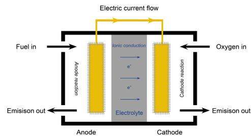
Figure 3.3: Schematic overview of a fuel cell
