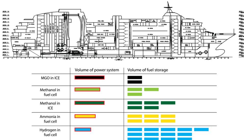
Figure 5.7: Visualization of the volumes of selected fuels and machinery on board of Ship B
