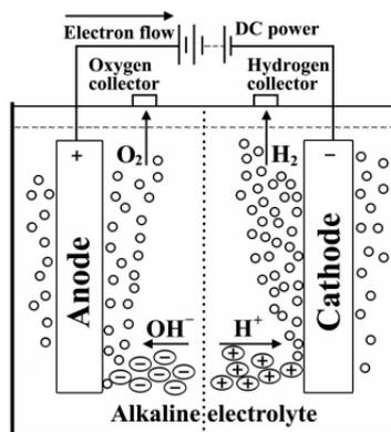
Figure 2.1: Schematic overview of electrolysis
