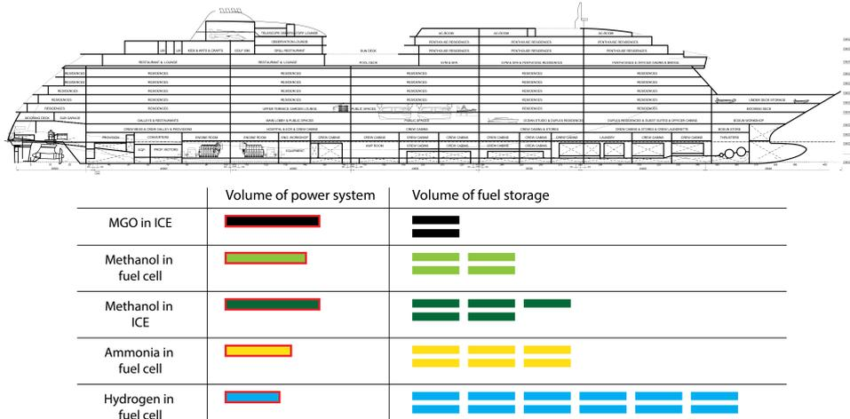
Figure 5.8: Visualization of the volumes of selected fuels and machinery on board of Ship C
