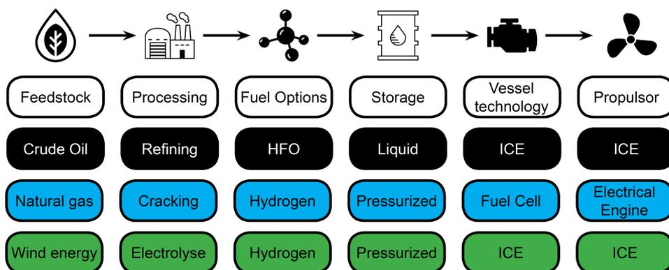
Figure 1.6: Energy chain from feedstock to propulsor with examples of HFO (black), hydrogen made from natural gas (blue) and hydrogen made from renewable energy (green)
