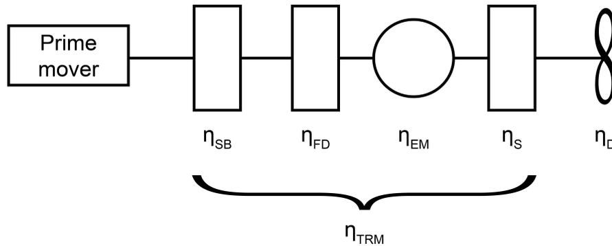
Figure 4.9: Propulsion power train sub-systems
