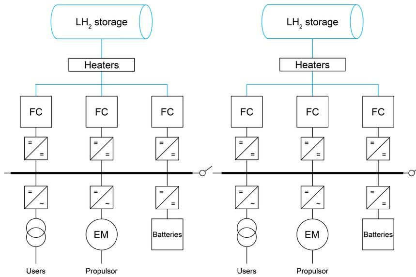
Figure A.1: Potential lay-out of liquid hydrogen power system
