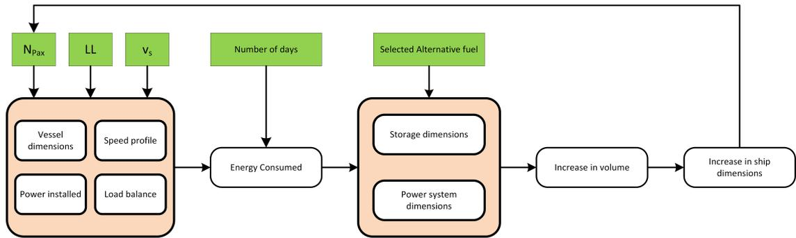
Figure 5.3: Schematic overview of the final design impact tool with iteration included
