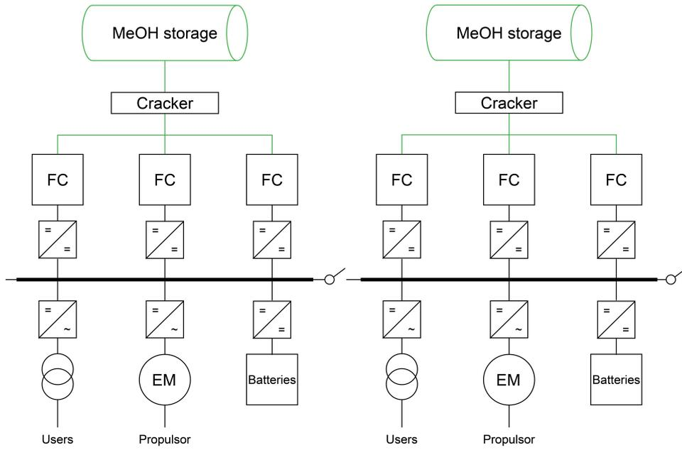
Figure A.3: Potential lay-out of methanol fuel cell power system
