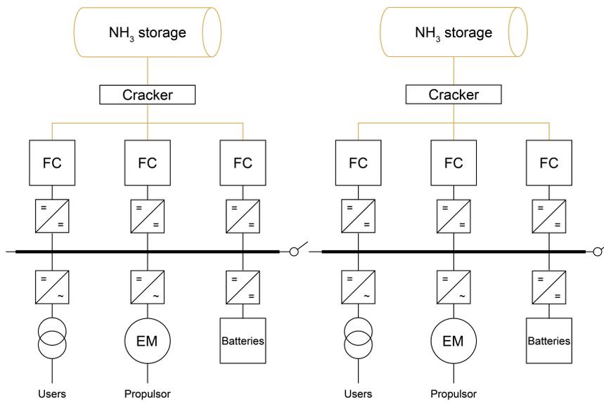
Figure A.2: Potential lay-out of liquid ammonia power system
