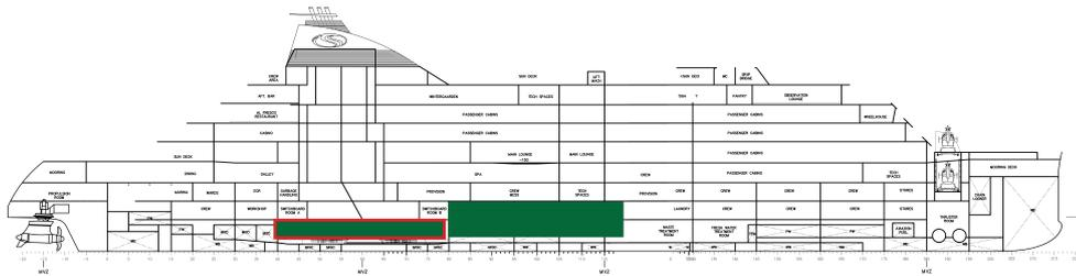
Figure C.3: Schematic GA for Ship A for the methanol ICE test case
