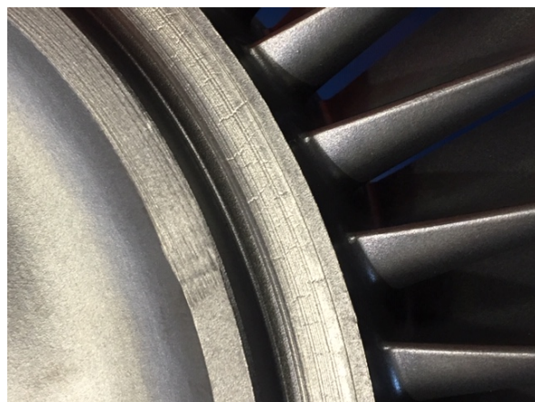
(b) Turbine wheel with initial cracking
