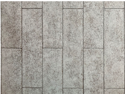
Wood wool cement board Cladding Underpasses roof 1982 - present day
