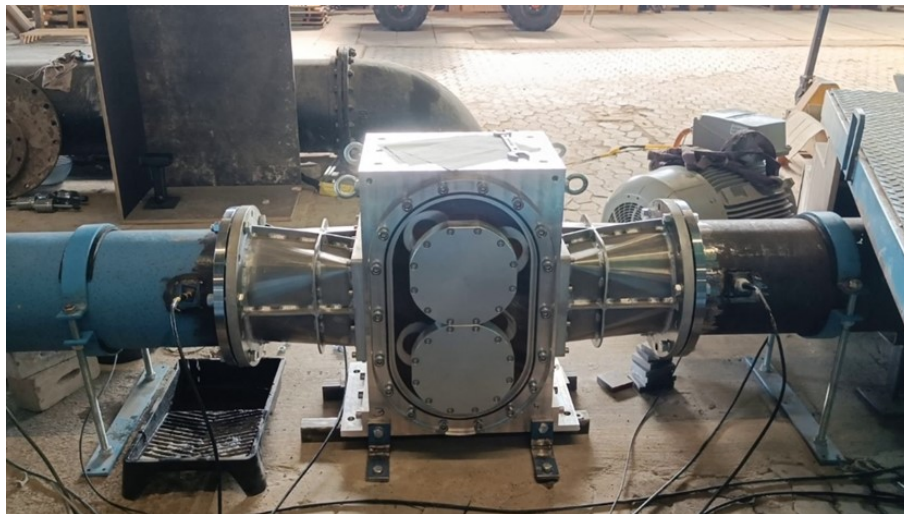
Figure 1: Side view of the PD-RPT unit during a wet test run at the TUB hydraulic lab.
