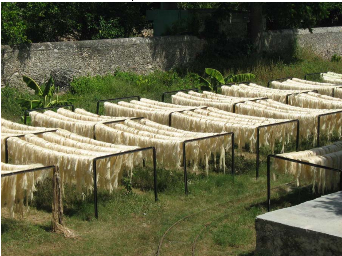
After washing, the fibres are dried Later they will be brushed and packed
