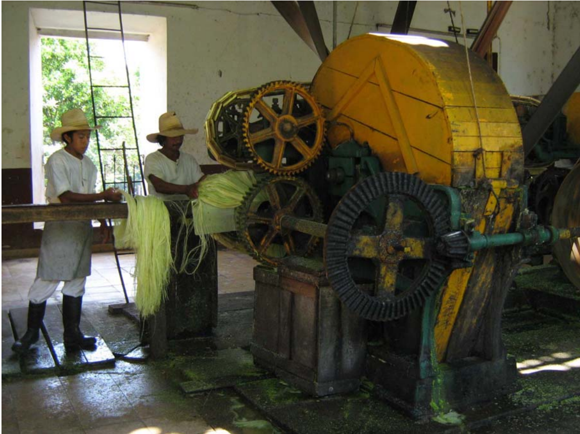
Decortication, leaves are crushed and beaten
