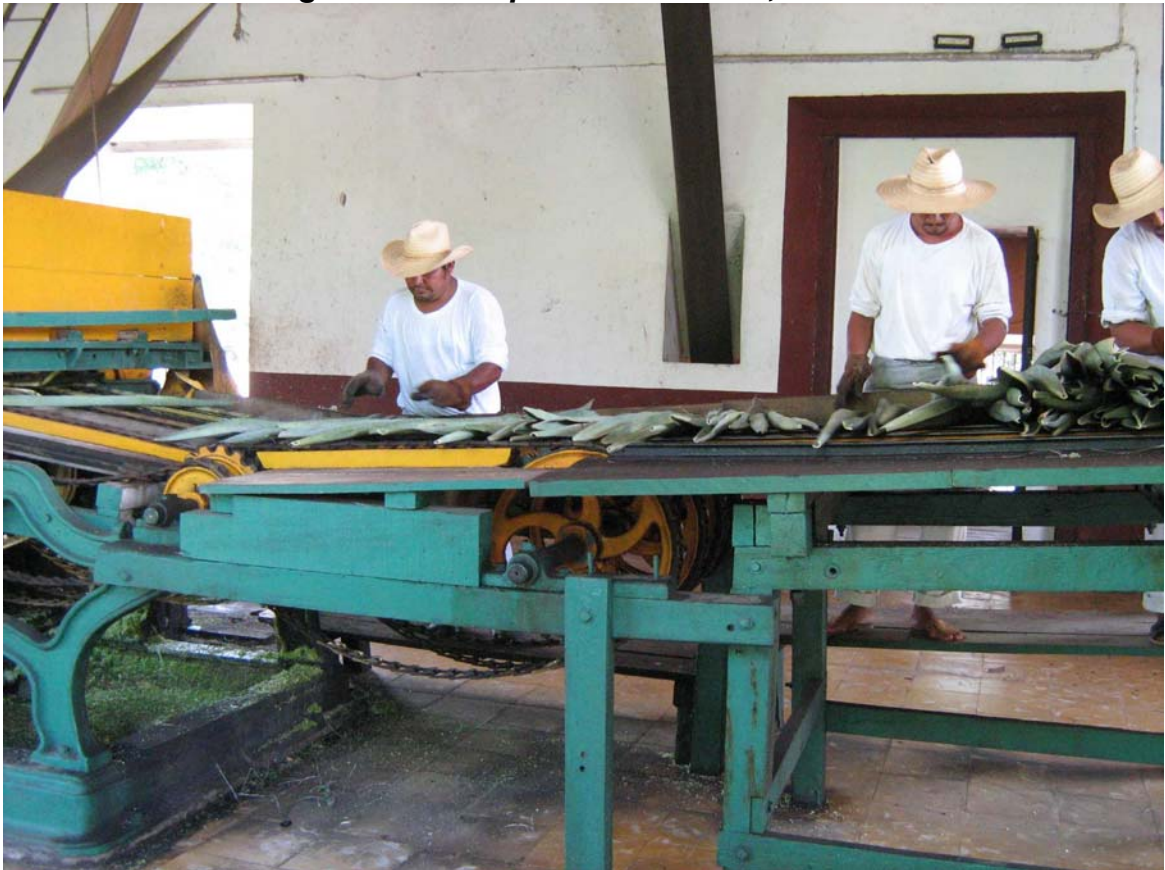
Decortication, leaves are crushed and beaten
