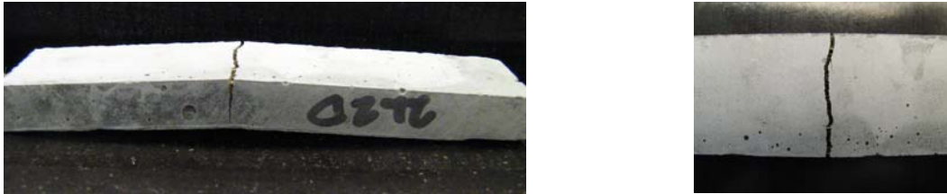
Figure 6.4: Larch fibre-crack-bridging in a sample tested under flexural load.
