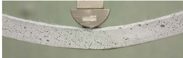
Figure 1.3: Example of multiple cracking and enhanced ductility of ECC [Boshoff 2007].
