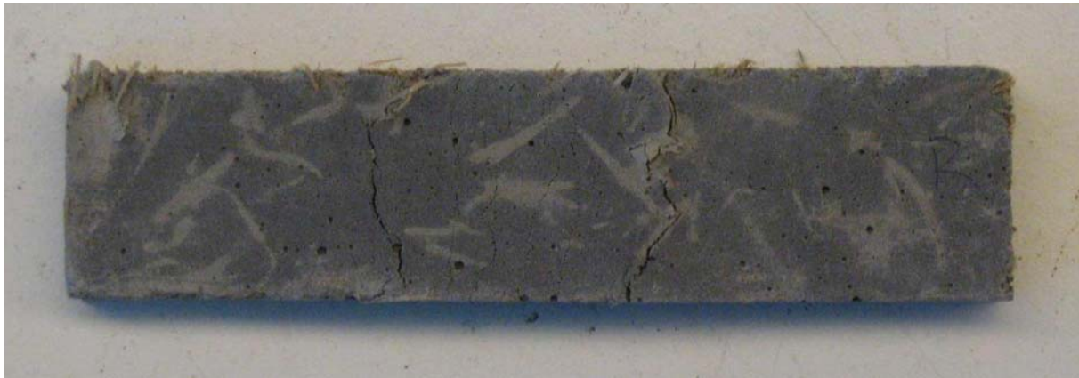
Figure 6.18: Multiple cracking of the samples under four-point bending load.
