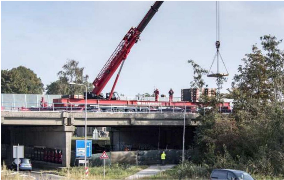
Figure 1. Collapse test being performed in October, 2016 on the Vechtbrug in The Netherlands (De Vries, Lantsoght, Steenbergen, & Fennis, 2022).
