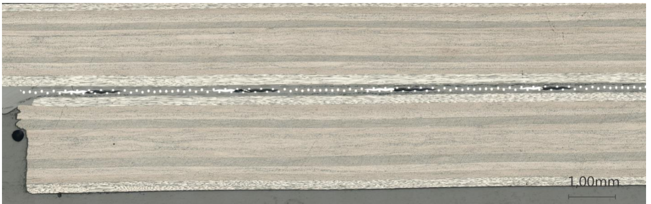
Figure A.7-2: Joint cross section microscopic view in the transversal direction of a joint welded with M200 HE
