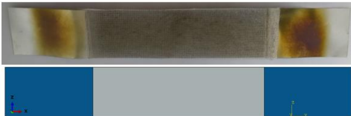
Figure 3.2-7: Continuous plate HE FEM modelling strategy. Laser cut plate HE (Top), FEM modelled HE (Bottom)
