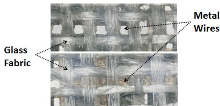
Figure 4.3-7: A005 wire size compared to glass fabric gap size (Top), C005 wire size compared to glass fabric gap size (Bottom)
