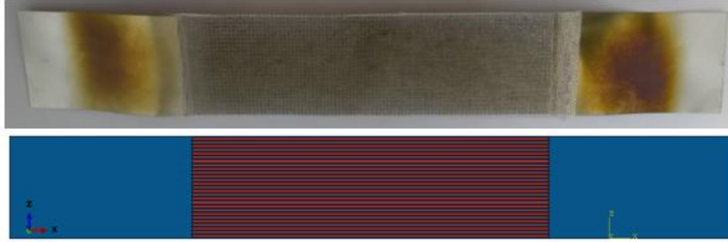
Figure 3.2-8: Longitudinal wires model HE FEM modelling strategy. Laser cut plate HE (Top), FEM modelled HE (Bottom)
