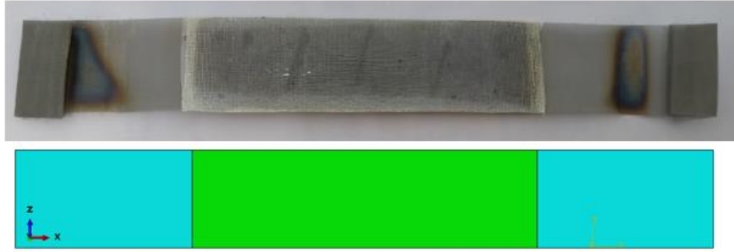
Figure 3.2-5: Continuous plate HE FEM modelling strategy. M200 HE (Top), FEM modelled HE (Bottom)
