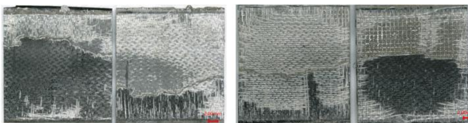
Figure 4.2-3: Failure surface of a joint welded with Porcher glass fabric used as a HE electrical insulator. M200 mesh HE(left), Concept_1_0_C005 HE (right).
