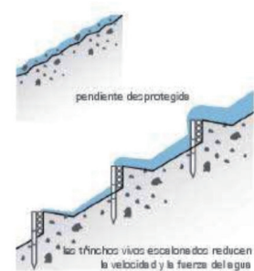
fig.72 Construction technique of slope stabilization. Source: Report of "Rehabilitar la Montana", municipality of Medellin.
