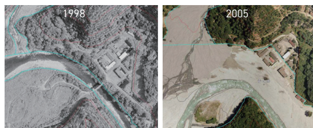
fig.45 Photos showing the damage caused by Typhoon in 2005, the power plant office and the dam was destroyed.
