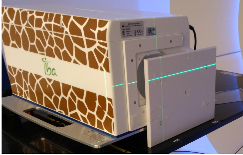
Figure 13: Setup for the WET uniformity measurements, the targets are placed in front of the IBA Giraffe.
