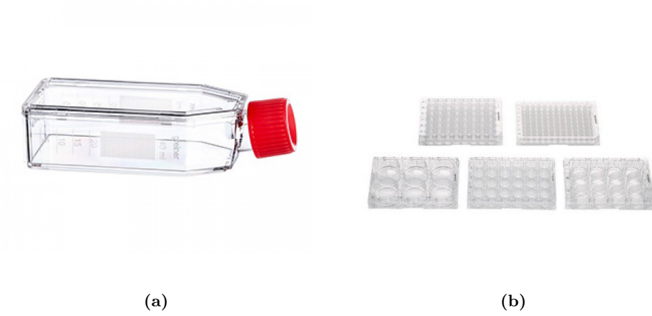
Figure 8: Cell cultureware often used in radiobiological experiments. (a) 50mL CELLSTAR T25 Flask. (b) Eppendorf multiwell culture plates
