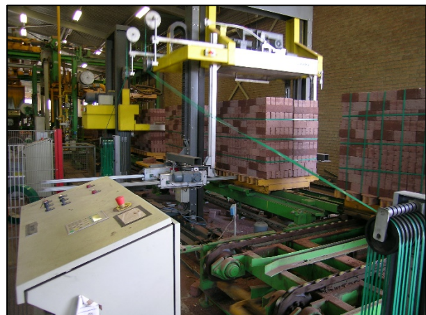
Figure 27. Packaging machine of bricks (KNB, 2020a).
