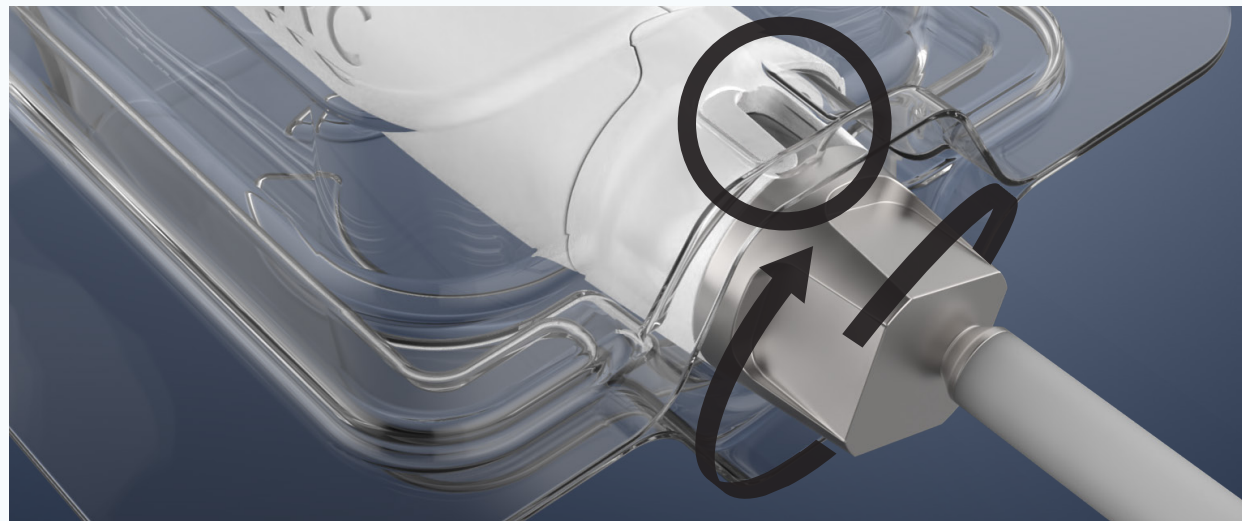
Figure 4.2 - 5 Visualisation of torque ridge reaching limit, collapsing due to rotation, and entire handpiece turning, indicating that the handpiece is assembled securely
