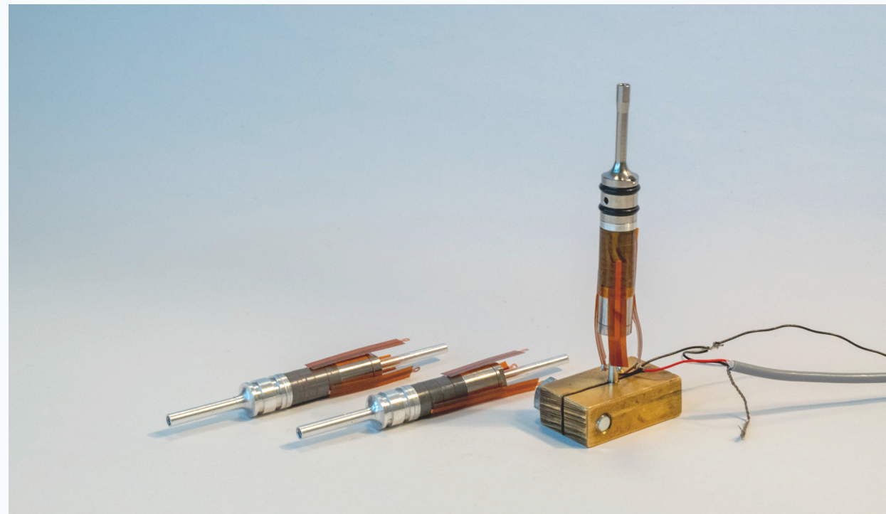
Figure 5.1 - 2 Sonotrode prototypes as used in a number of ultrasound performance tests
