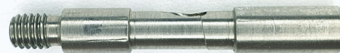
Figure 5.1 - 6 Tested transmission shaft student design showing a crack due to added load from stroke amplification (at a stress concentration)
