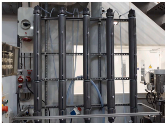
Fig. 3. Laboratory scale Denutritor® columns. (Source: Author).
