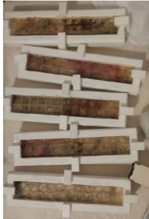
Example of warping without clamped during preparation (left) and individual clamps for tensile testing (right).
