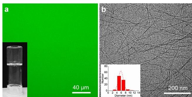
**Figure 2.** a) Confocal images of the gel networks, inset in a) is photograph of the gel sample; and b) cryo-TEM image of the gel fibers, inset graph is the diameter distribution of the fibers. Samples are prepared from  $[\mathbf{H}] = 20$  mM,  $[\mathbf{A} + \mathbf{A}^-] = 120$  mM (30 mol%  $\mathbf{A}^-$ ),  $[\mathbf{A-FL}] = 30$  μM,  $[\mathbf{Hoechst 33342}] = 20$  μM, and seeds consisted of 1.0 mM **NGs**.
