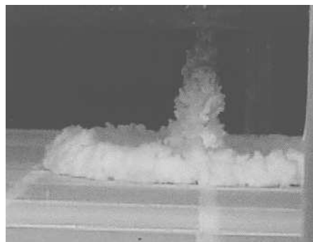
Figure 4.4: A density current in still water. After Boot (2000)
