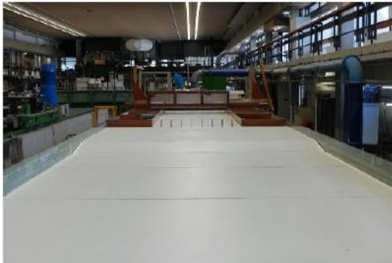
Figure 2.19: An overview of the experimental setup with a lateral expansion, depth increase by a false bottom and grid elements (Van de Zande, 2018).
