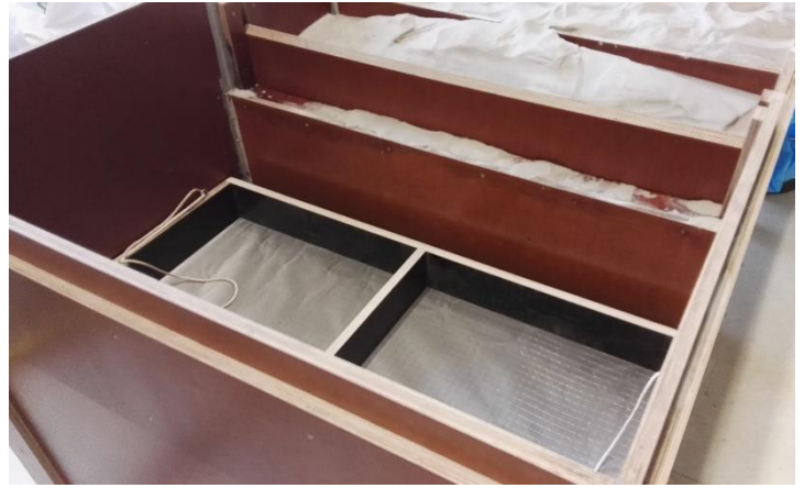
Figure C.4: Sieve at the end to collect the eroded sand
