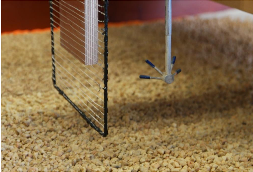
Figure 3.8: Measuring the velocities using ADV and bubble frame.
