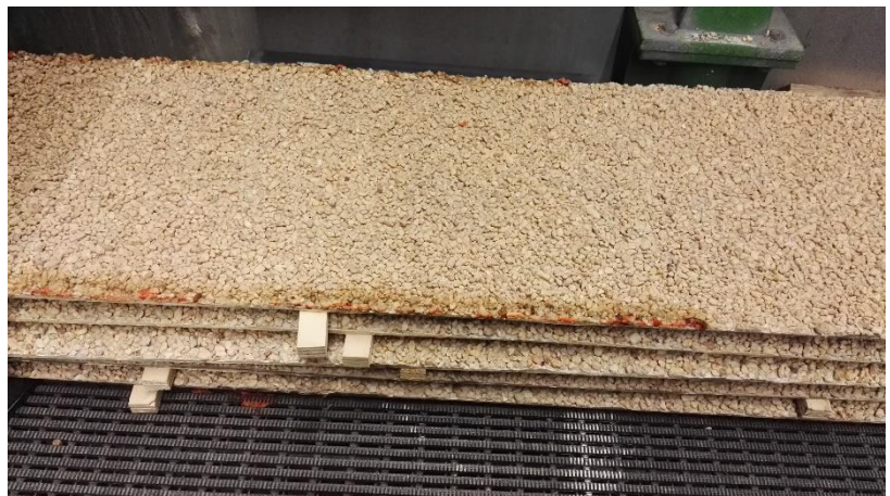
Figure C.2: The plates with roughness (glued gravel)
