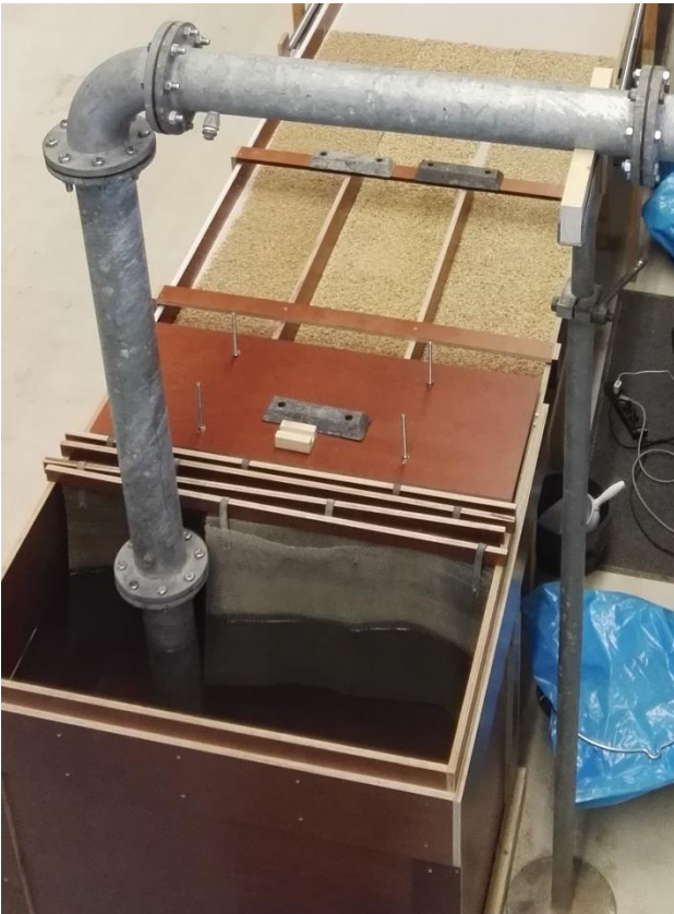
Figure C.5: The inlet section with asymmetrical pump and several meshes to smoothen the flow
