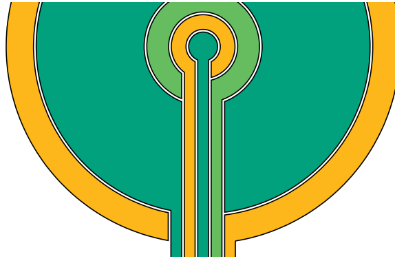
Figure 2.31: Zoomed-in illustration of mask 1 of a circular sensor with 5 bottom contacts. Different colours are used to differentiate between the individual contacts
