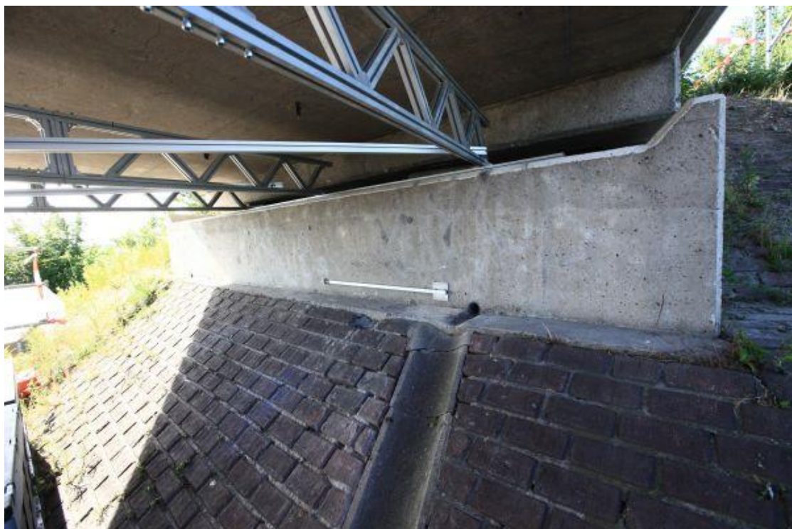
Fig. 18: Position of reference LVDT to measure influence of temperature and humidity. Picture showing support 5.
