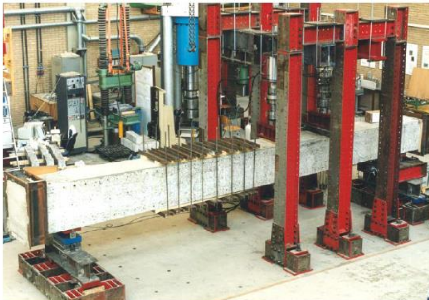
Fig. 12: Testing of beams with ASR-damage in the Stevin Laboratory (den Uijl and Kaptijn 2002). Photograph by J. A. Den Uijl, used with permission.
