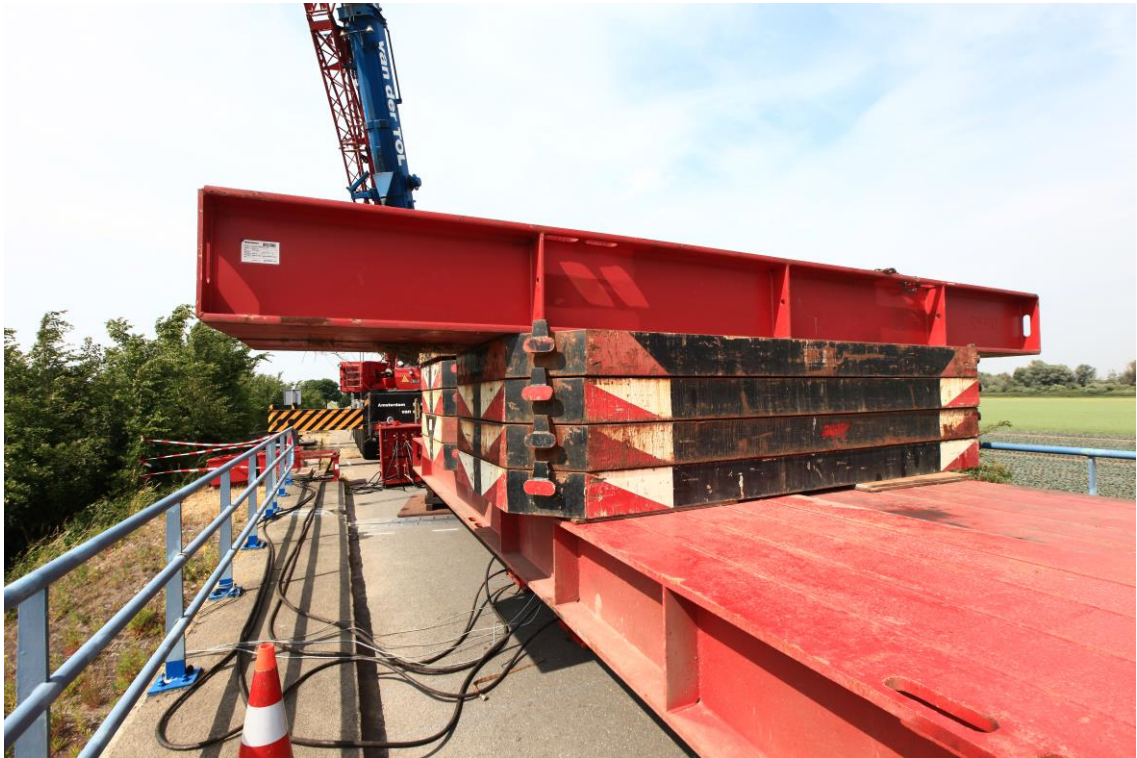
Fig. 21: Setup of the load used on viaduct Zijlweg.
