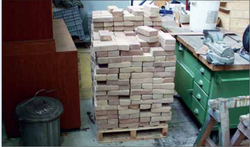
The newly fired fifty/fifty bricks containing 50% brick granulate and 50% clay.
