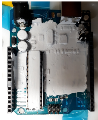
Figure 13: Application of a removable, high-emissivity fluid to the ArduinoUNO.
