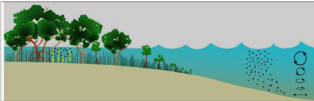
Figure 3-10 Transmission through mangrove forest and sedimentation (University of Waikato, 2016)
