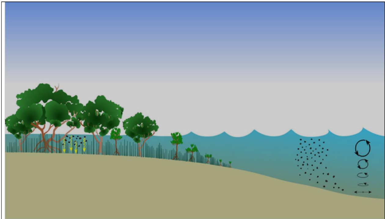
Figure A- 2 Transmission through mangrove forest and sedimentation (University of Waikato, 2016)
