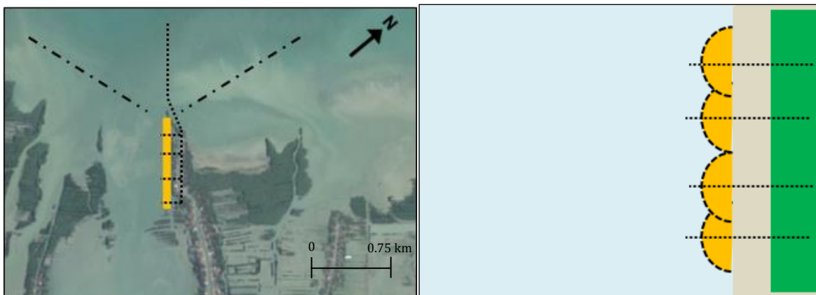
Figure 7-8 Possible pipe line approach and discharge configuration from land (top view) – full coastline
