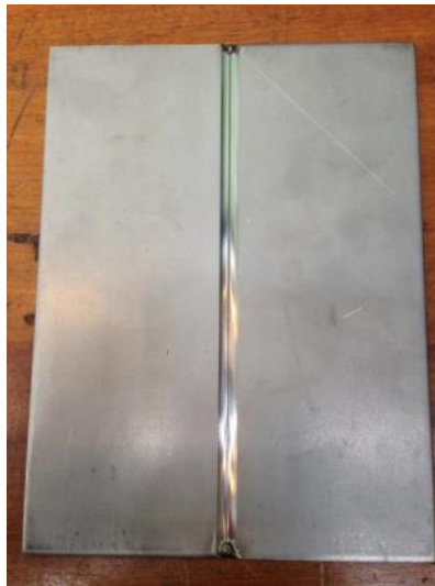
Figure 3-1 The tack welded workpiece in the butt welding.
