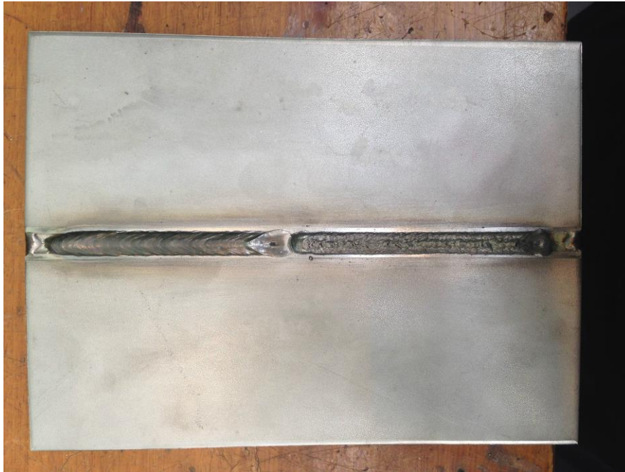
Figure 4-27 The appearance of weld beads for the cases of Ar (left) and Ar+3.3% CO 2 (right).
