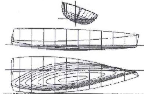
**Figure 3:** Underwater asymmetry of a heeled hull
