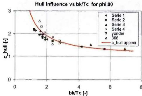
**Figure 2:** Hull influence coefficient for different keel series
