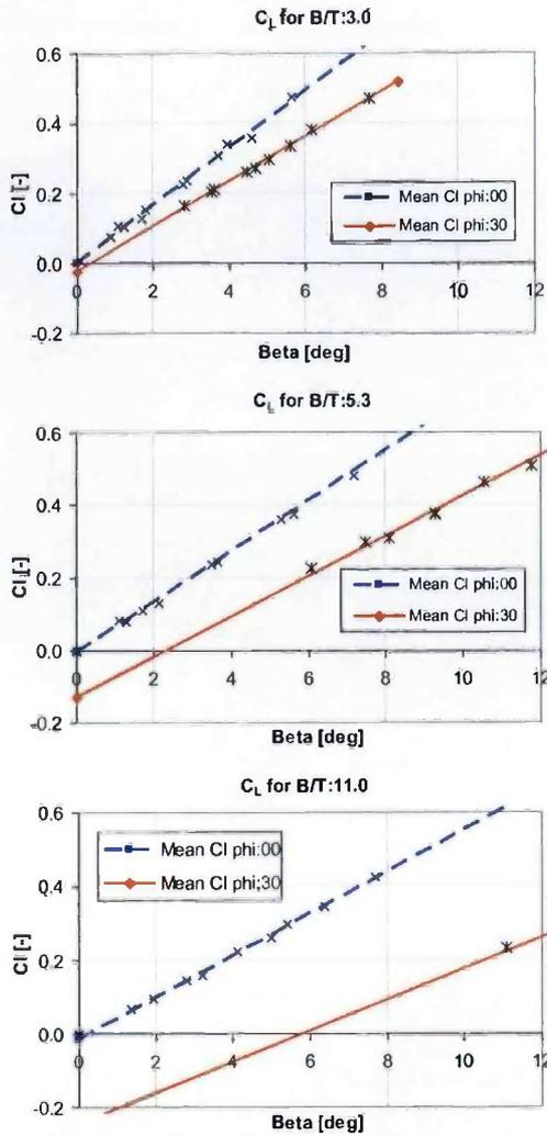
Figure 4: Lift coefficients for zero and  $30^\circ$  heel
