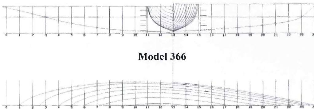
**Figure 5:** Lines plan of the model hull #366 used for the experiments
