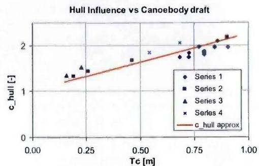
Figure 1: Hull influence coefficient for standard DSYHS appendages
