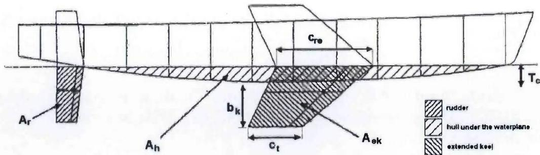
Figure 1: Definitions in the Extended Keel Method
